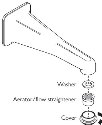
1 There is an aerator/flow straightener located in the end of the spout. To remove this unscrew and remove the cover.
